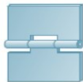
Hinge and bearing supporting axial thrust and radial load
