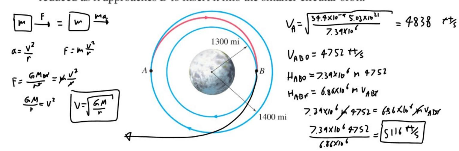
$$V_{B} = \sqrt{\frac{39.4 \times 10^{-9} 5.03 \times 10^{11}}{6.36 \times 10^{6}}} = 5022 \text{ ft/s}$$
