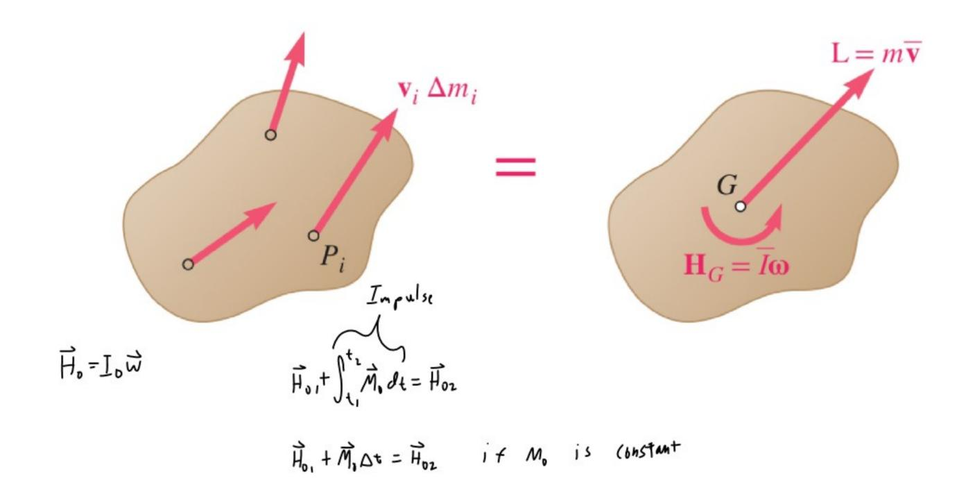
The rotor of an electric motor has a mass of 25 kg, and it is observed that 4.2 min is required for the rotor to coast to rest from an angular velocity of 3600 rpm. Knowing that kinetic friction produces a couple of magnitude 1.2 N·m, determine the centroidal radius of gyration for the rotor.
