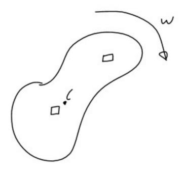
A 200-kg flywheel is at rest when a constant 300 N·m couple is applied. After executing 560 revolutions, the flywheel reaches its rated speed of 2400 rpm. Knowing that the radius of gyration of the flywheel is 400 mm, determine the average magnitude of the couple due to kinetic friction in the bearing.
