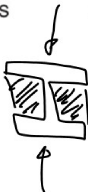
Stage 3: Roughing horizontal and vertical rolls
