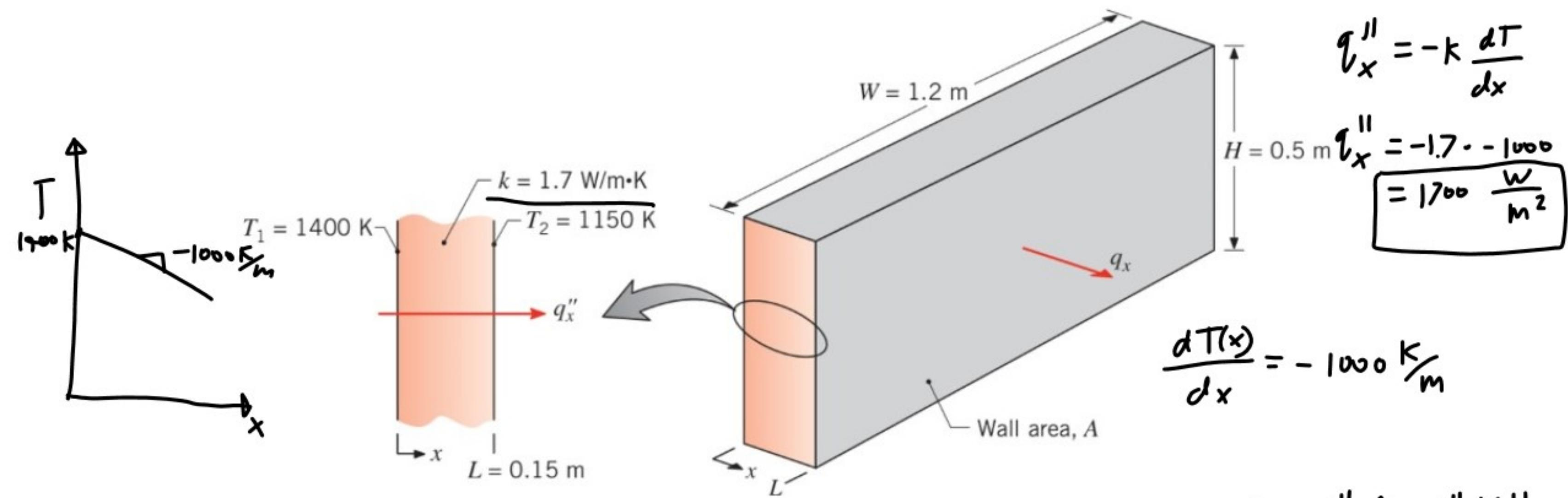
Consider the fireclay brick wall of Example 1.1 that is operating under different thermal conditions. The temperature distribution, at an instant in time, is  $T(x) = a + bx$  where  $a = 1400 \text{ K}$  and  $b = -1000 \text{ K/m}$ . Determine the heat fluxes,  $q''_x$ , and heat rates,  $q_x$ , at  $x = 0$  and  $x = L$ . Do steady-state conditions exist?
