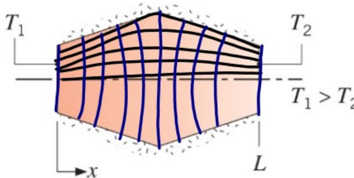
If the properties remain constant and no internal heat generation occurs, sketch the heat flux distribution,  $q''(x)$ , and the temperature distribution,  $T(x)$ . Explain the shapes of your curves. How do your curves depend on the thermal conductivity of the material?
