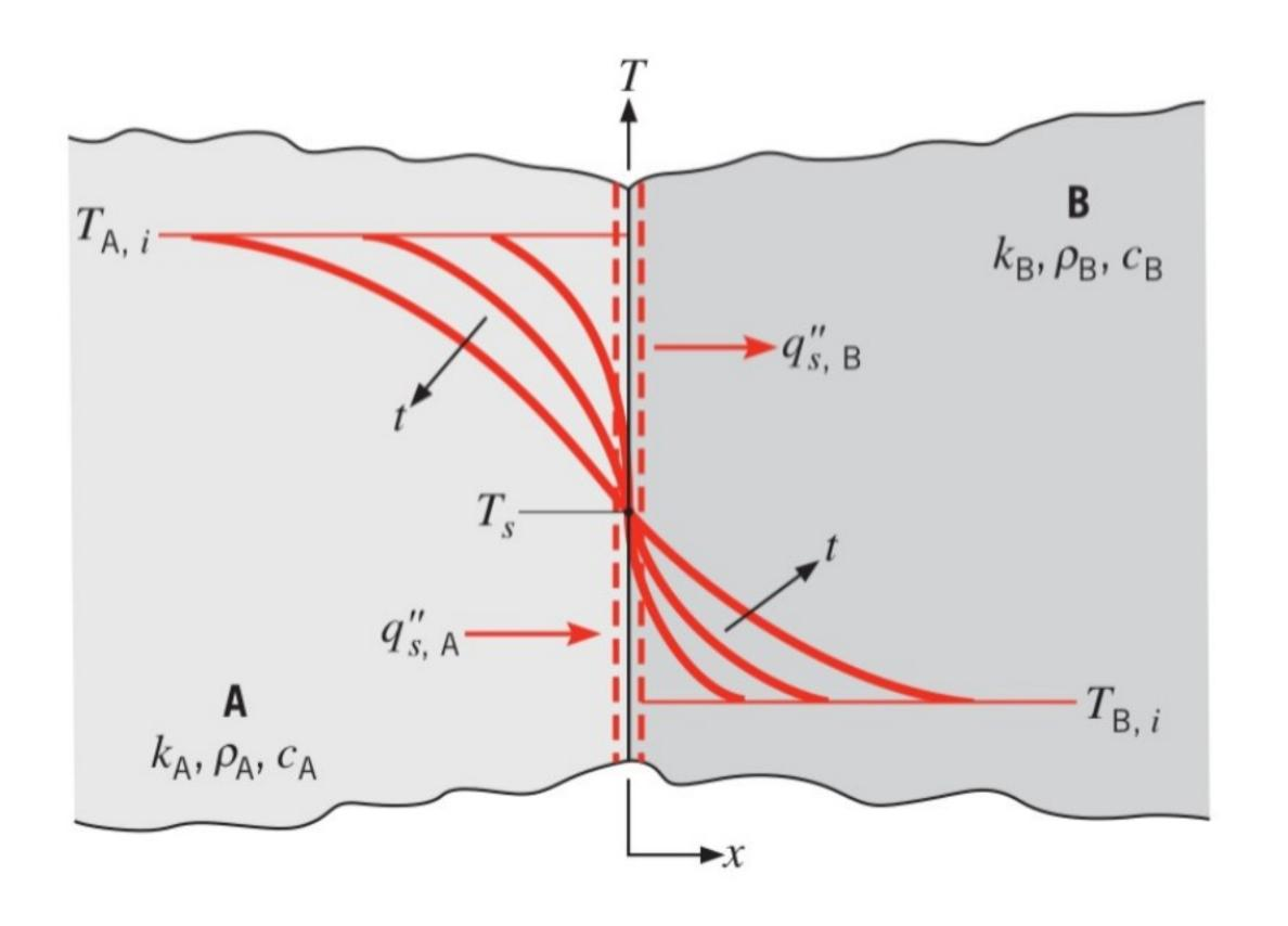
$$\frac{2''_{SA} = 2''_{SB}}{-K_{A}(T_{S} - T_{A:})} = \frac{K_{B}(T_{S} - T_{B:})}{\sqrt{\pi a_{B}t}}$$
