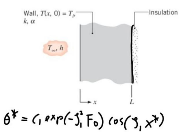
For a particular wall, case 1, the temperature at  $x = L_1$  after  $t_1 = 100$  s is  $T_1(L_1, t_1) = 315$ °C. Another wall, case 2, has different thickness and thermal conditions as shown.
