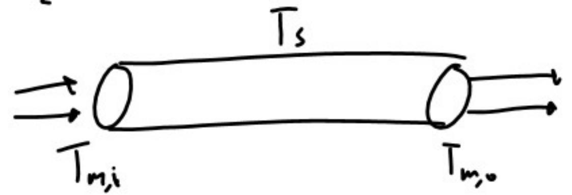
**8.20** Engine oil flows through a 25-mm-diameter tube at a rate of 0.5 kg/s. The oil enters the tube at a temperature of 25°C, while the tube surface temperature is maintained at 100°C.
