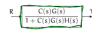
Figure block.2: a block diagram with the corresponding closed-loop transfer function block, derived in Example intro.block-1.
