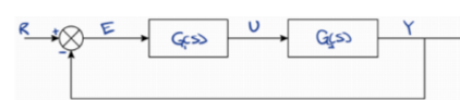
Figure error.1: unity feedback block diagram with controller G_1(s) and plant G_2(s) .
