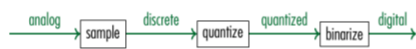
Figure 06.1: the operations required to convert an analog to a binary digital signal.
