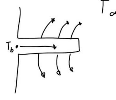
3.99 Turbine blades mounted to a rotating disc in a gas turbine engine are exposed to a gas stream that is at  $T_{\infty} = 1200^{\circ}\text{C}$  and maintains a convection coefficient of  $h = 250 \text{ W/m}^2 \cdot \text{K}$  over the blade.
