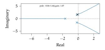
Notice that double-clicking the locus yields a data cursor that gives the complex coordinate and corresponding gain! For instance, at the coordinate -0.10 + j1.61, the gain is 0.67. Therefore, to place a closed-loop pole at this location, we would choose K = 0.67.
