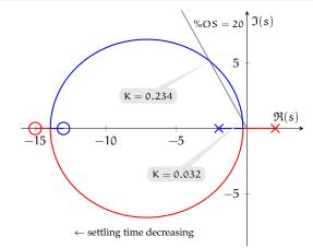
From the figure, we can see that when the gain is either K = 0.032 or K = 0.234, according to the second-order approximation, the %OS is 20. We prefer the latter because of our requirement to minimize the settling time, which decreases as the closed-loop poles move leftward. Now we must find the closed-loop transfer function, which can be found as follows.
