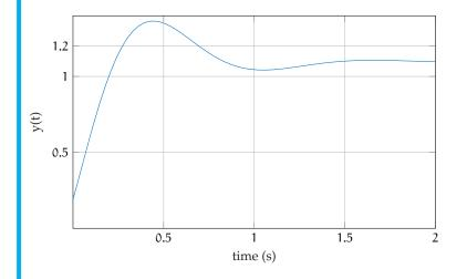
Note that the steady-state error is nonzero (which we can't really do anything about). Looking back at the root locus plot, we see that as the gain increases from here, the percent overshoot should decrease. We iterate the gain to obtain K = 0.35. The final closed-loop step response is shown, below.
