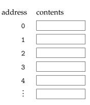
When storing a multi-byte number, we use the bigendian convention: the MSB is stored at the lower address. The littleendian convention stores the MSB at the higher address.
