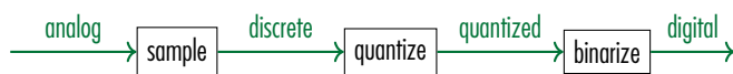
Figure 06.1: the operations required to convert an analog to a binary digital signal.
