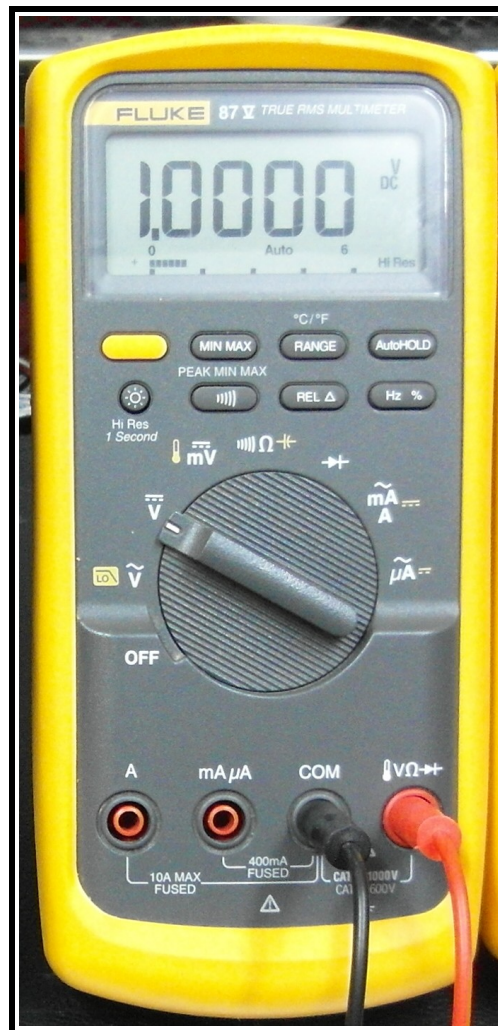
Figure 02.4: the front panel of a Fluke multimeter, connected in high-resistance mode.
