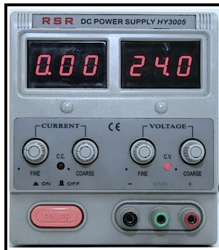
Figure 02.1: the front panel of the HY3005 dc power supply.
